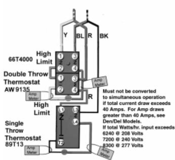
Note: Amperage will only be indicated while electricity flows through a wire.
